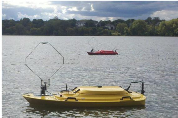
Fig. 1. The robotic systems used in field experiments. The 2-meter boats were designed to track invasive fish autonomously. Each is equipped with wireless communications, directional antenna used as bearing sensors, a navigation suite, and computing hardware. Our algorithm was implemented on this system and was shown to localize targets to within small uncertainty.
