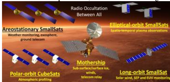
Figure 2: MOSAIC multi-platform measurement concept
